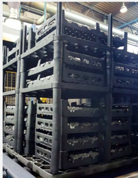
Fig. 1: Production batch stacked in cast baskets and cast base trays
