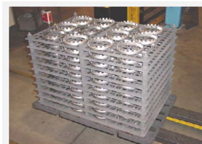
Fig. 1: Fully loaded CFC fixture with internal ring gears, 10-layers (3-dimensional), 120 parts (1)
