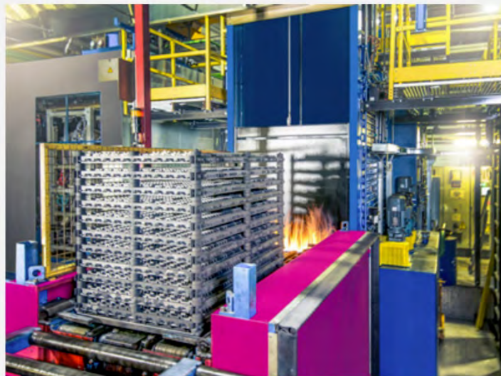
Fig. 3: Production batch comprising CFC workpiece fixtures, 11-layers, in front of the furnace door (Source: HEAT Holding)
