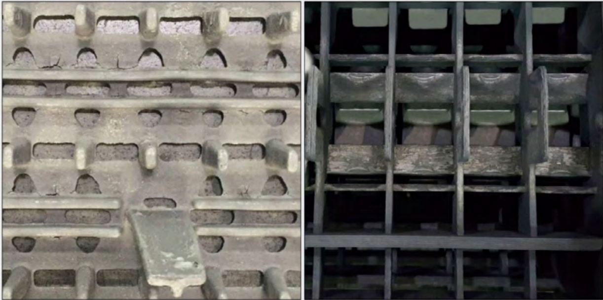
Fig. 4: Component loading in the cast basket and the CFC layer (not to scale)
