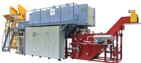
Continuous furnaces with online quenching
