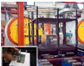
PhoenixTM system in TUS measurement jig. Inset shows data logger being placed into thermal barrier.
